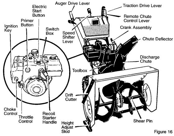
Auger Drive Lever – Starts and stops the auger and impeller (snow gathering and throwing)
